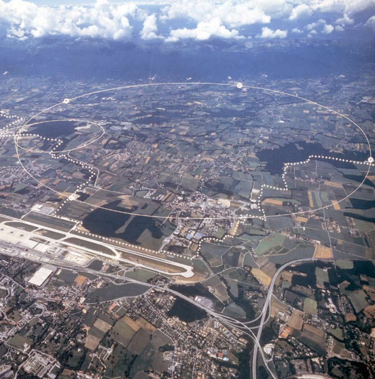
Aerial view of the CERN site just outside Geneva. The large circle shows the line of the LEP tunnel, 27 km in circumference, the small circle shows the SPS tunnel, 7 km in circumference. The crossed line indicates the border between France and Switzerland.
